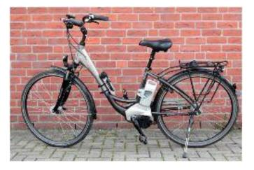
Driving offers assistance up to 25 km / h (license free). The battery is conveniently charged using the charger.
