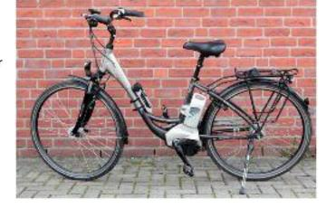
Driving offers assistance up to 25 km / h (license free). The battery is conveniently charged using the charger. Note: The permissible total weight for our electric bikes is 130 kg. The minimum size is 150 cm.
